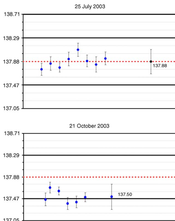
Fig. 2. Intraday reproducibility of ^{960}\text{U} isotopic measurements without bracketing. Major grid lines are at 3‰ spacing.
